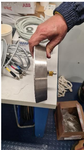
Figure 8-2 - Insert for pressure sensor
