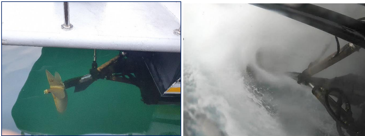
Figure 8: Goldwing’s surface piercing propeller in port (left) and during high-speed transit (right)
