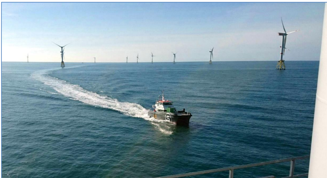
Figure 1: CTV approaching a monopile in an offshore wind farm (source: DW-ShipConsult)
