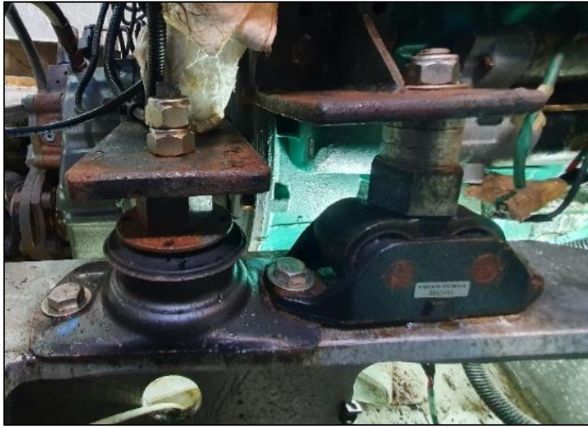
Figure 33: Example of an elastic engine mount. Picture taken on GW.
