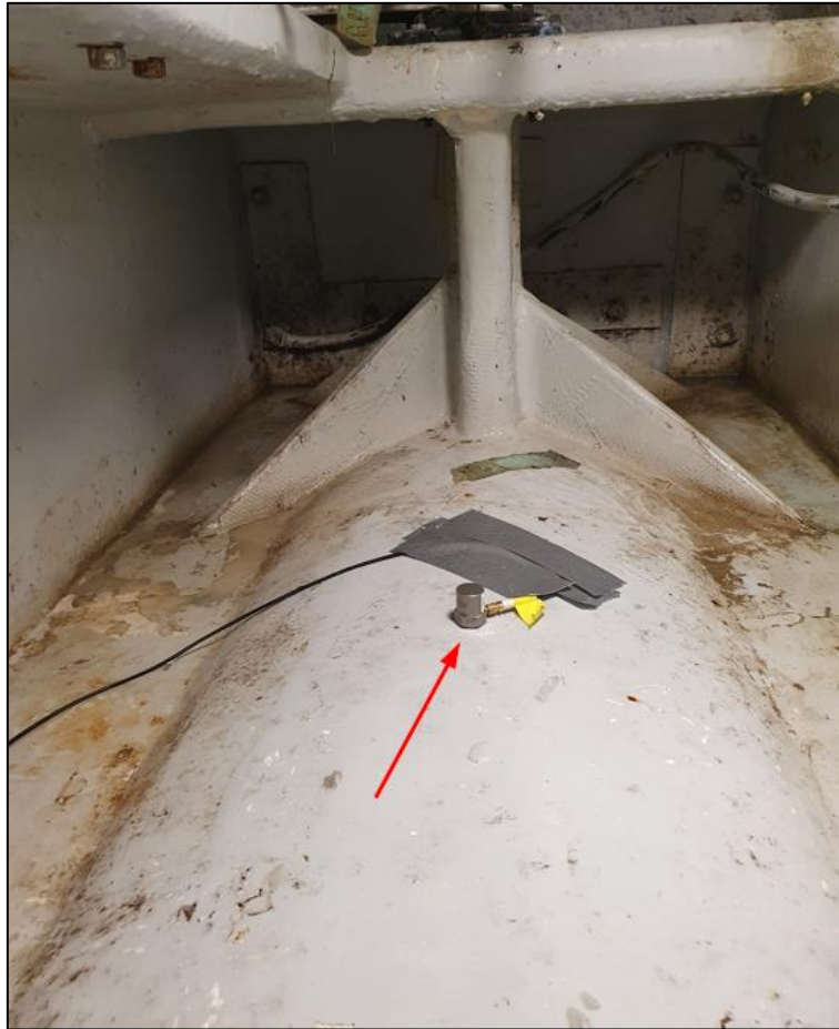
Figure 22: SBN sensor above propeller of 4EW
