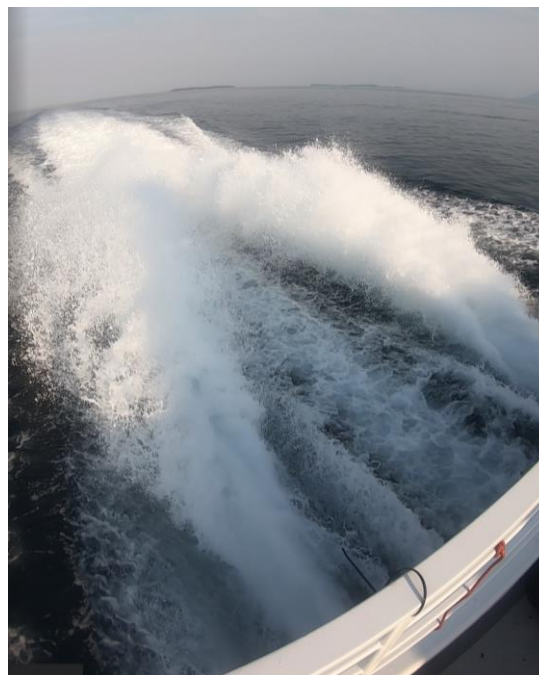
Figure 72: waterjets hitting the surface in the wake of the boat
