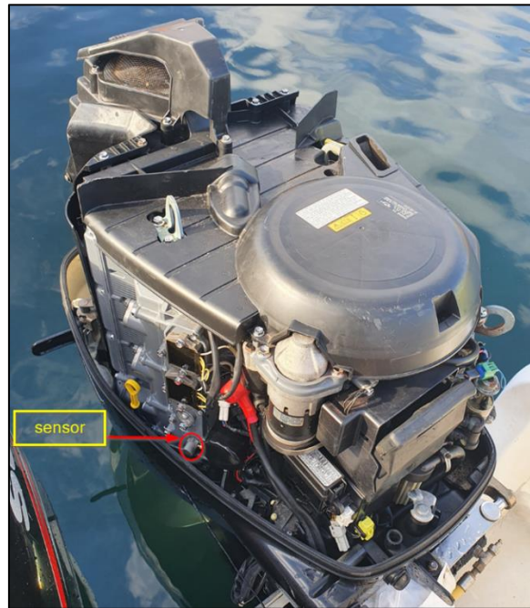
Figure 47: SE: Sensor Position at Engines; PS Engine Shown
