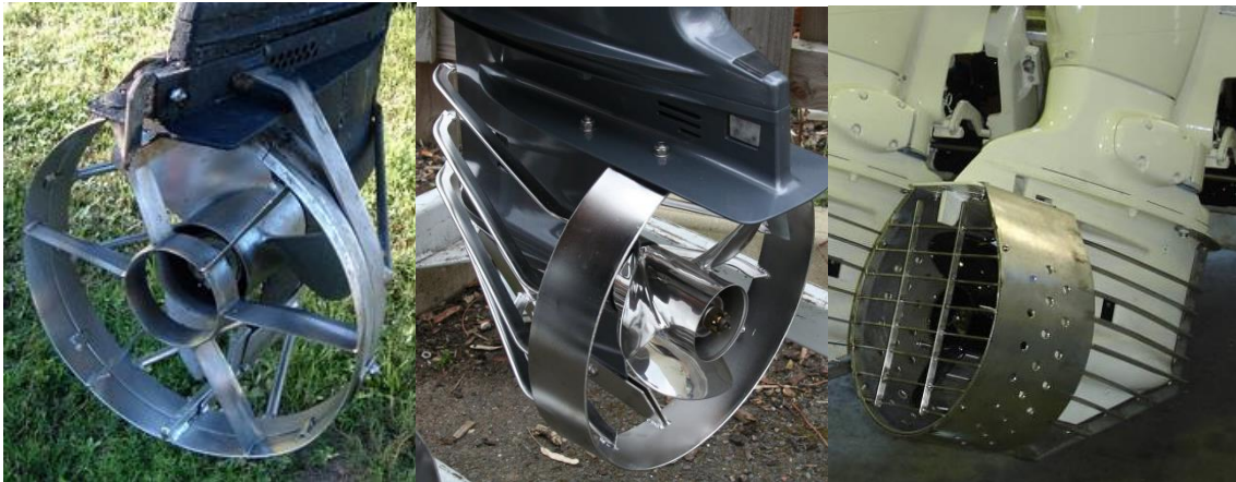
Figure 5-4: Ring / cage combination guards (left: PropGuard, middle: BH Fabrications, right: Holton Marine Ltd.)
