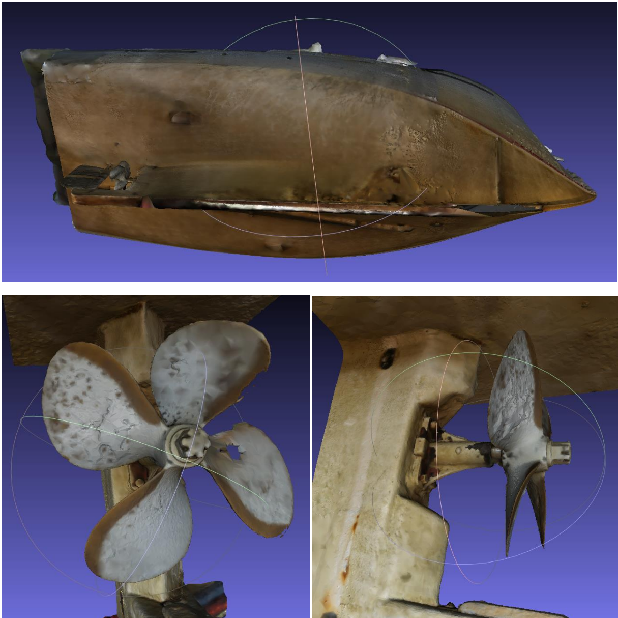
Figure 4-1: 3D photogrammetry scan geometries of the Bay Bliss hull (top) and propeller (bottom)
