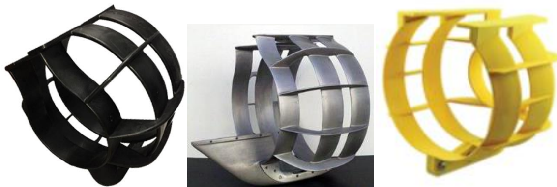
Figure 5-5: Kort nozzle guards (left: PropGuard, middle: Thustor, right: GH Marine)
