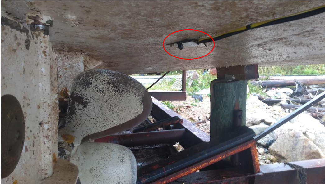
Figure 3-2: Pressure sensor location (in red circle) on This Is It 1.
