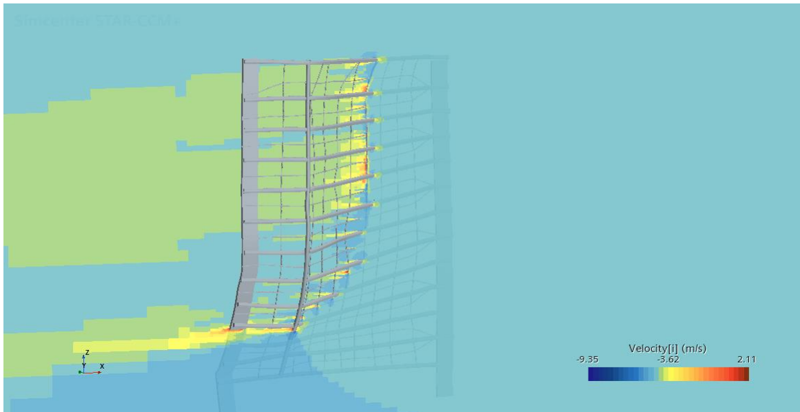
Figure 4-23: Open water propeller velocity contours
