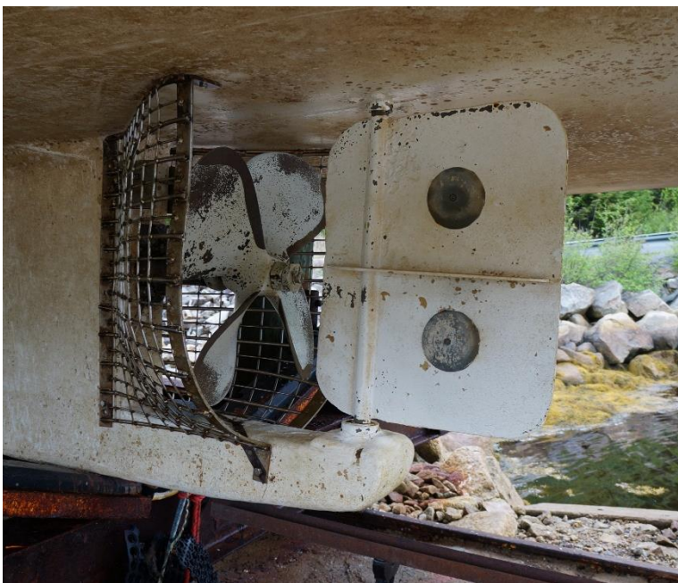
Figure 2-2: Port-Aft view of propeller, cage, and rudder on This Is It 1.
