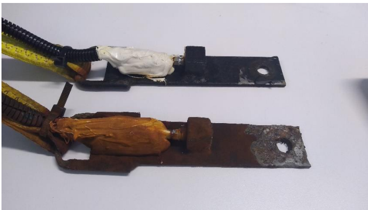
Figure 3-3: Pressure sensor damage
