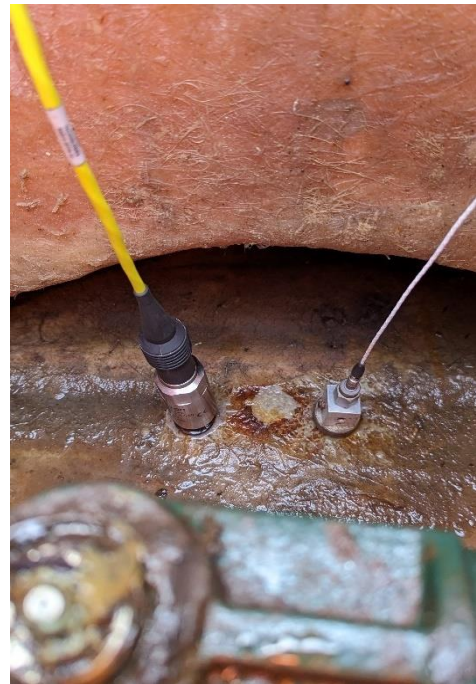
Figure 5-4 Two accelerometers mounted on hull above fishing boat propeller. Mounted Left: CBM 4-20 mA Wilcoxon Accelerometer. Mounted Right: IEPE reference accelerometer.
