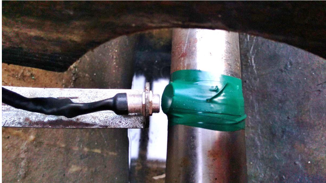
Figure 5-6 Close up of Hall Effect Tachometer and triggering magnet.
