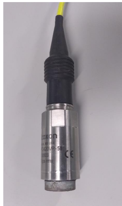
Figure 3-5 (Left) CBM 4-20 mA Wilcoxon Accelerometer (yellow cable) mounted on hull above a fishing boat propeller. (Right) IEPE Accelerometer with magnetic base installed.
