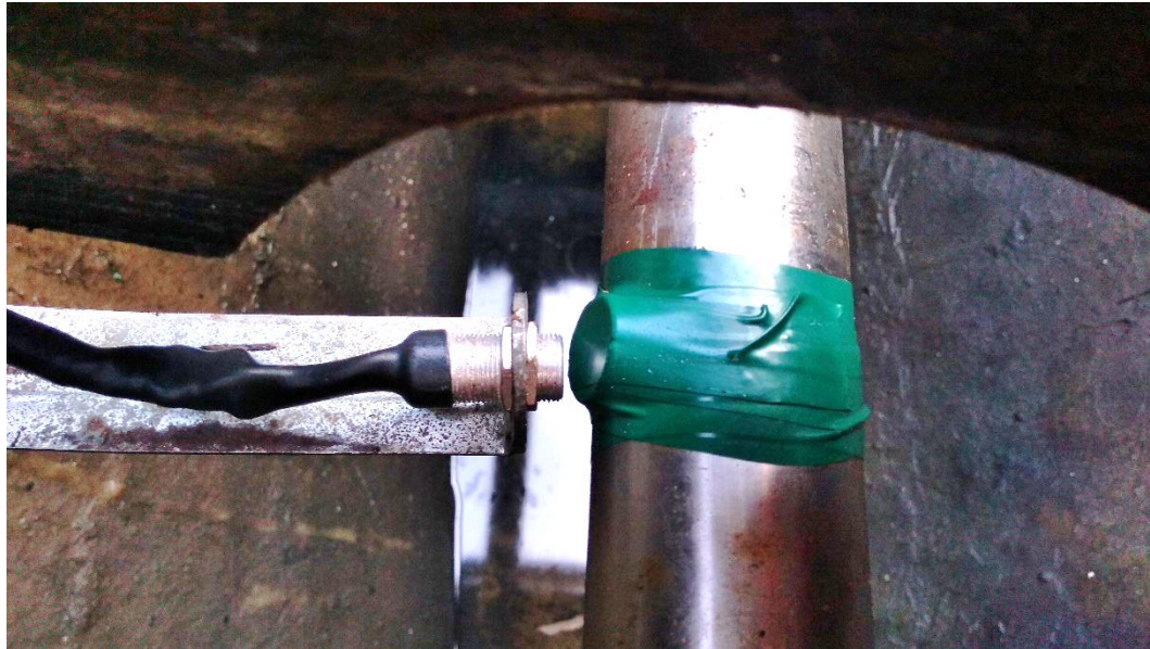
Figure 3-4 Close up of Hall Effect Tachometer and triggering magnet (attached with green electrical tape to propeller shaft).
