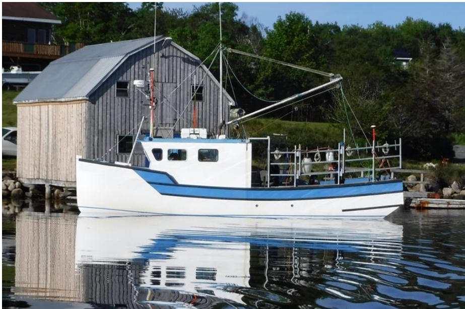
Figure 1-1 Example of the class of small marine craft known as Cape Islanders
