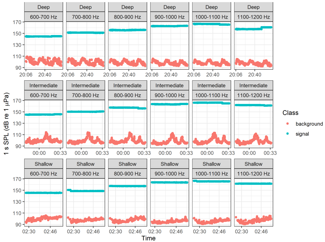
Figure C-4. OSM (1 m hydrophone) measured signal and background sound pressure level (SPL) as a function of range during the propagation loss (PL) experiment.
