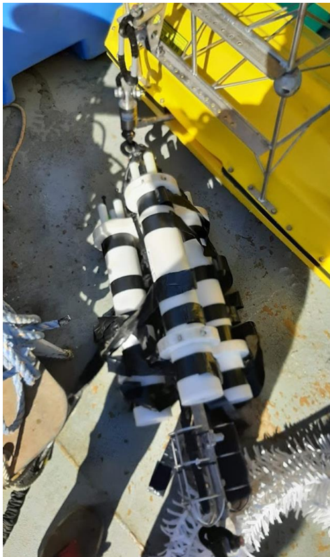
Figure 10. The top-most AMAR from mooring 240A showing vortex shedding elements added for the February 2021 trial. Four pieces of 5 cm duct tape were required for the AMAR tubes, and a 5 cm hairy fairing wrap for the vectran cables. The black open-cell foam flow shield can be seen on the right hand hydrophone. The untreated left hand hydrophone is visible inside the steel protective cage.
