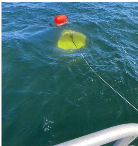
Figure 21. The 72-inch sea anchor deployed from the Celtic V in July 2021. Photo by Graham Warner, JASCO Applied Sciences.
