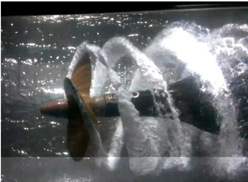
Figure 1. Visualization of cavitation shedding from the tips and face of a propeller (photo from: https://www.youtube.com/watch?v=SEvxngv-dkY ).
