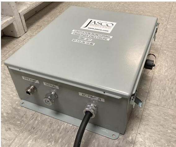
Figure 9. JASCO Observer enclosure located in the steering gear compartment. Photo by Art Cole.
