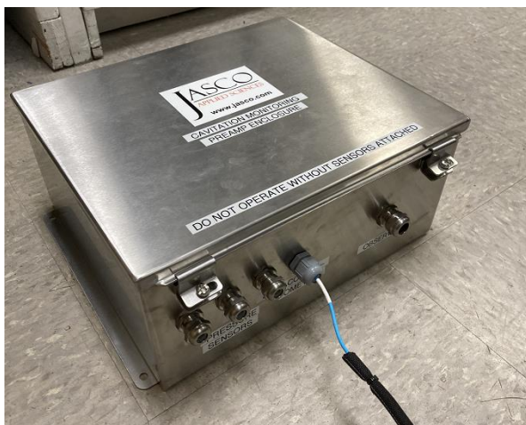
Figure 8. Preamplifier conditioning enclosure located in M/V Ferbec’s aft peak. Photo by Art Cole.
