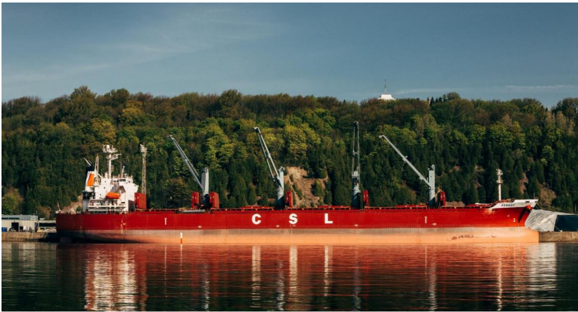
Figure 2. Picture of the M/V Ferbec , a 187.5 m, 49500 deadweight tonnage (dwt) bulker operated by CSL.
