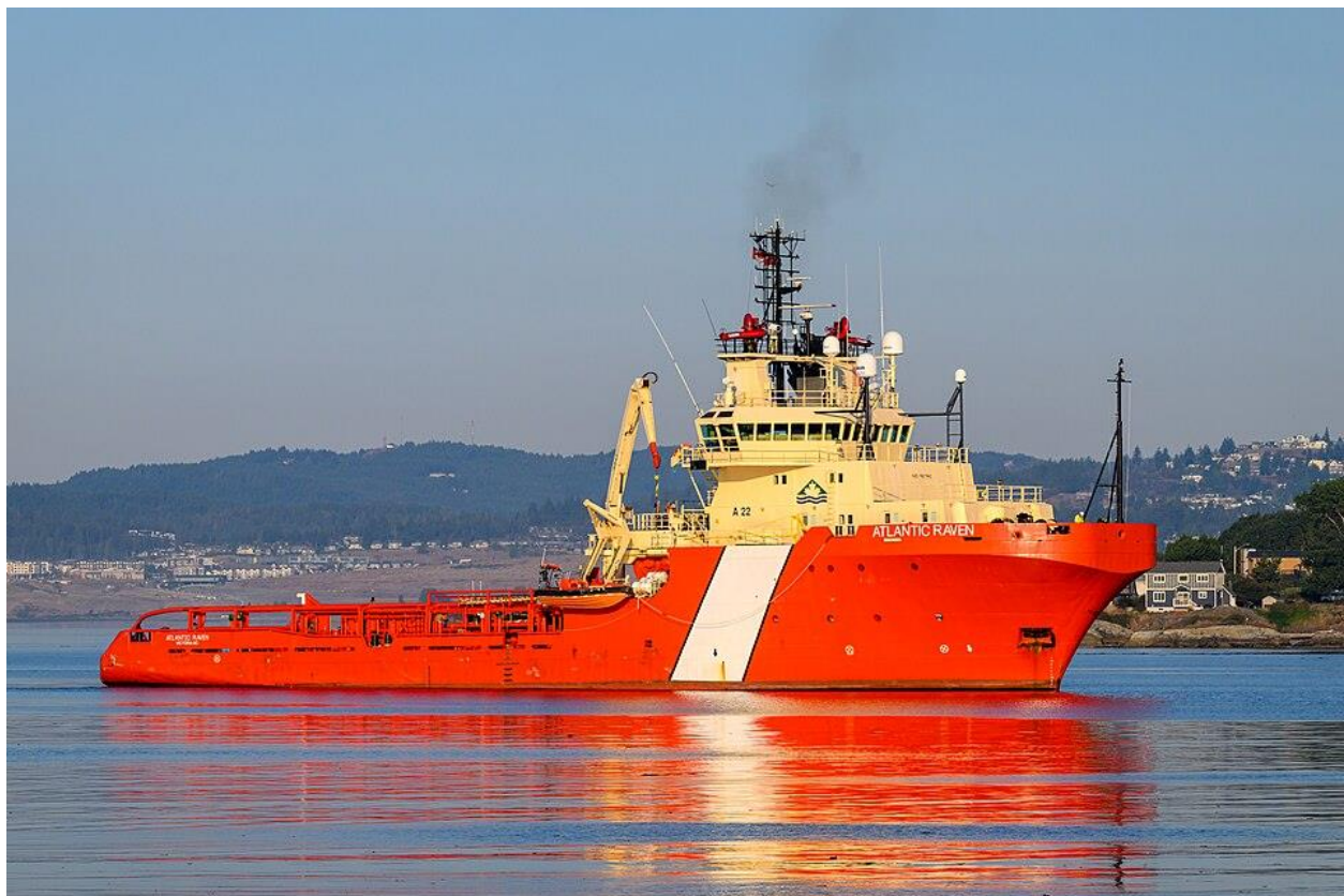
Figure 2 Example of an anchor handling tug supply (AHTS) vessel with sufficient bollard pull to act as an ETV. [Pictured: Atlantic Raven , bollard pull 162 tonnes]. Image Source .
