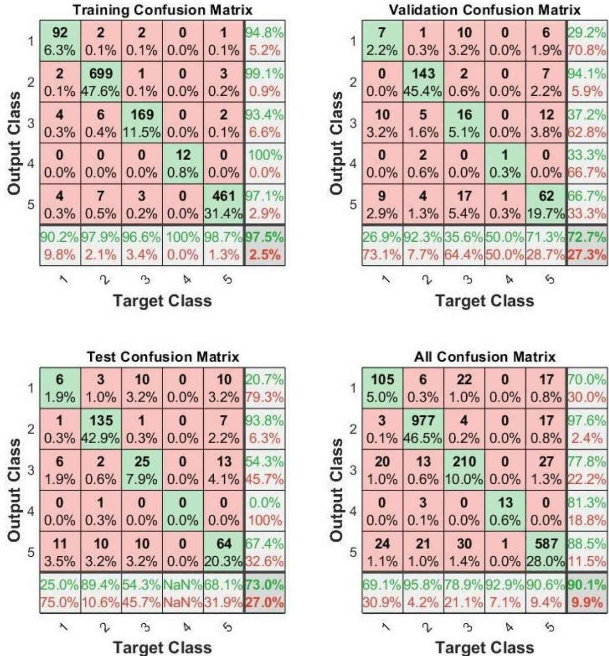
Figure 6-9 – The Confusion matrices resulted from the implementation of Neural Network algorithm on data using four attributes of the first 50 peaks of noise signals and four attributes of the first 25 peaks of vibration signals
