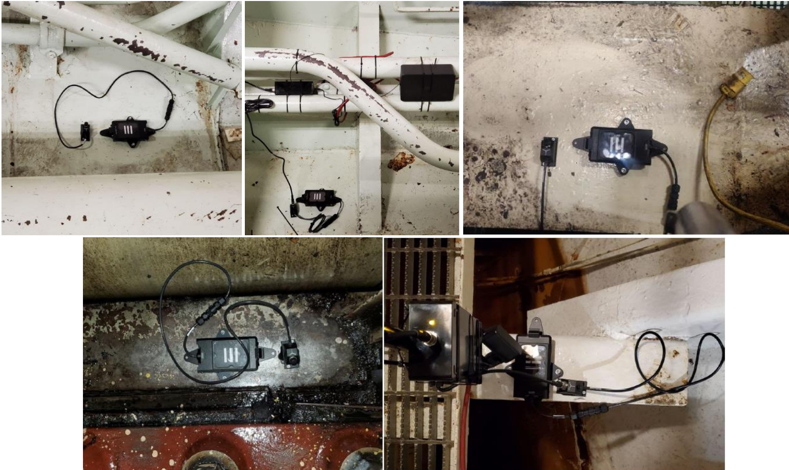
Figure 4-16 - Example sensor placement. Top left: Kinetix vibration sensor, End 2 propeller shaft; Top middle: Kinetix vibration and Tascam noise sensor, End 1 propeller shaft; Top right: Kinetix vibration sensor, End 2 gearbox; bottom left: Kinetix vibration sensor, End 1 engine; bottom right: Kinetix vibration sensor, End 2 steering compartment.
