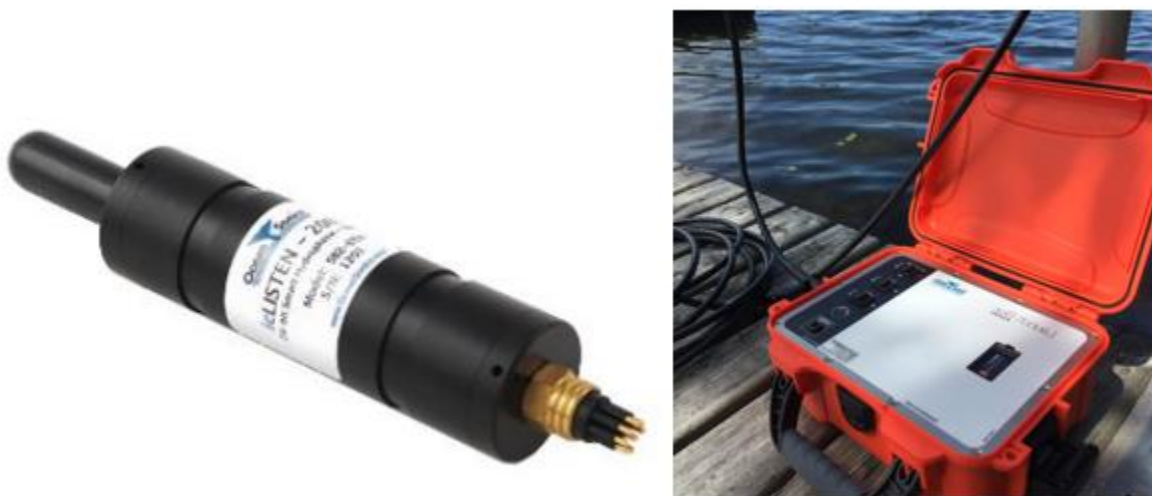
Figure 4-11 - icListen hydrophone unit (left) and launch box (right)
