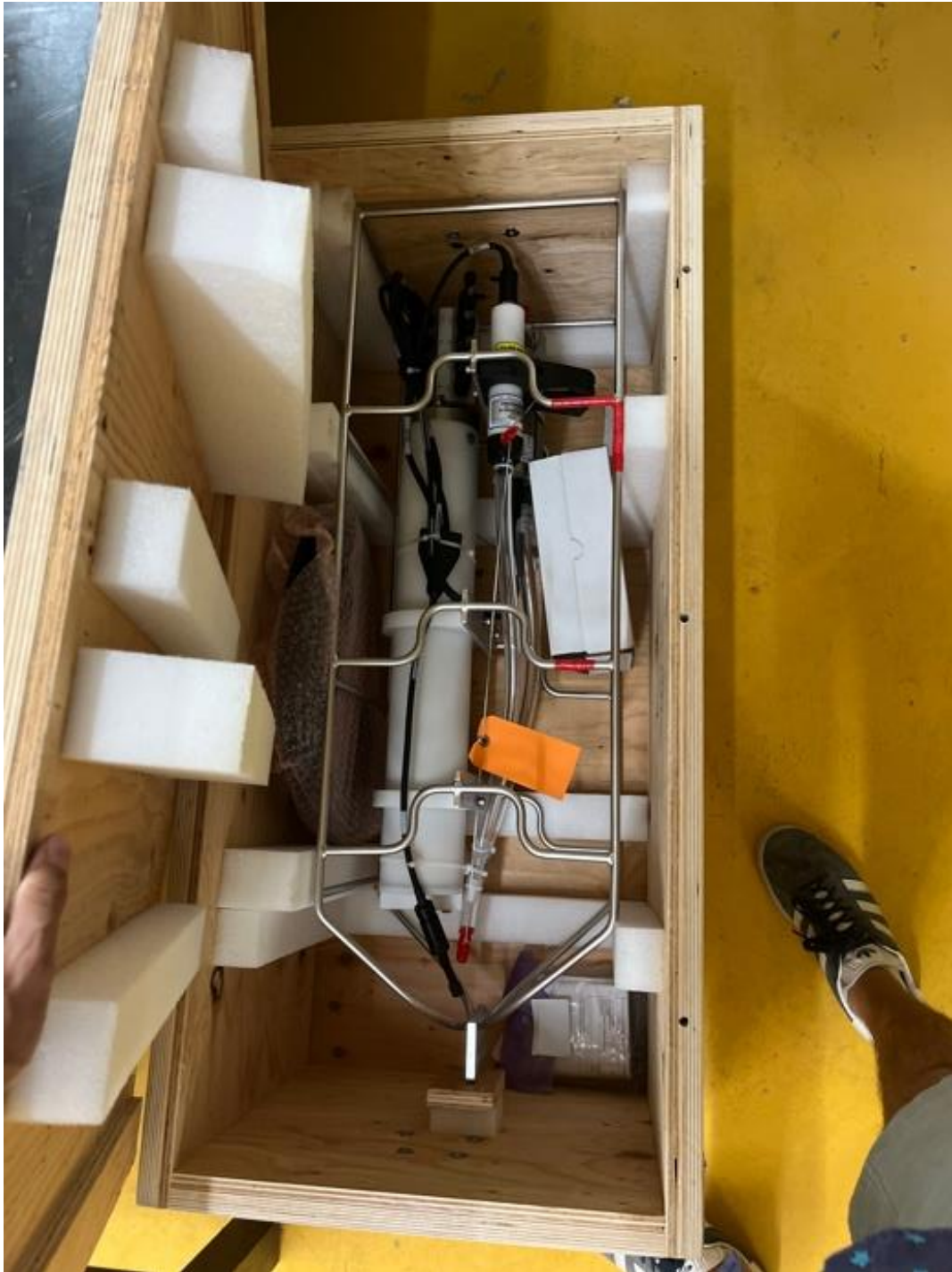
Figure 2-5 Conductivity, Temperature, and Depth (CTD) sensor
