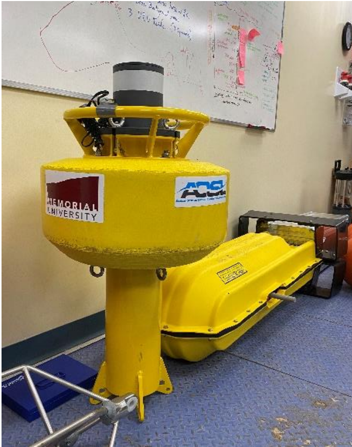
Figure 2-4 Surface Data Collection Buoy with Wi-Fi
