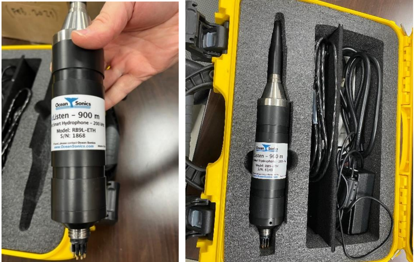
Figure 2-3 Digital Hydrophone: IcListen with Ethernet output
