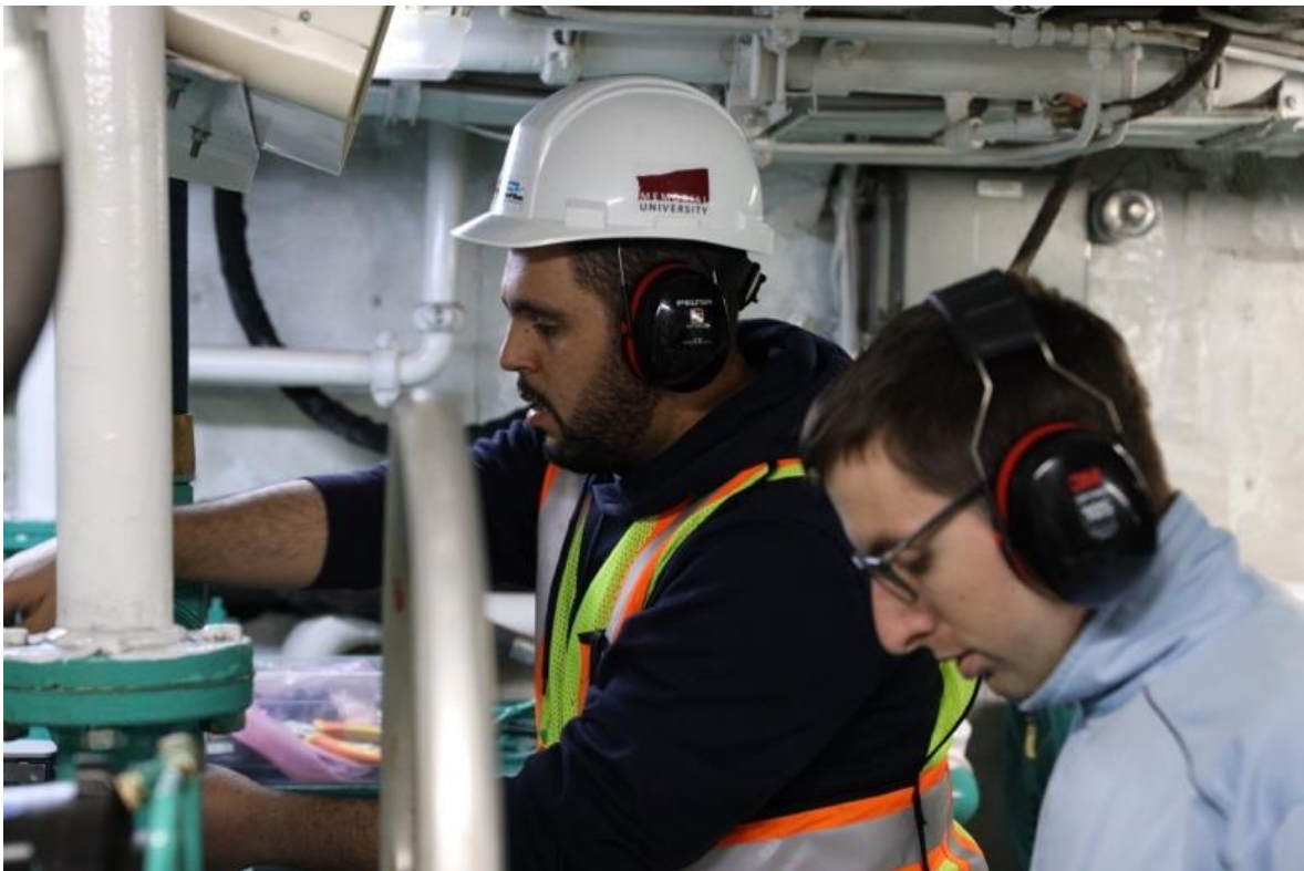
Figure 2-12 Structure-borne noise data acquisition in the vessel's steering room
