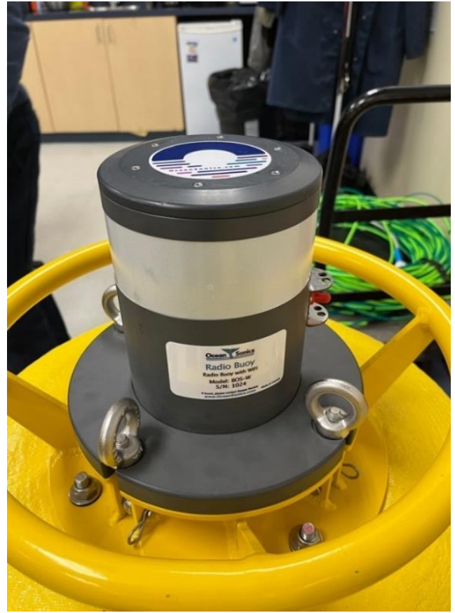
Figure 2-4 Surface Data Collection Buoy with Wi-Fi
