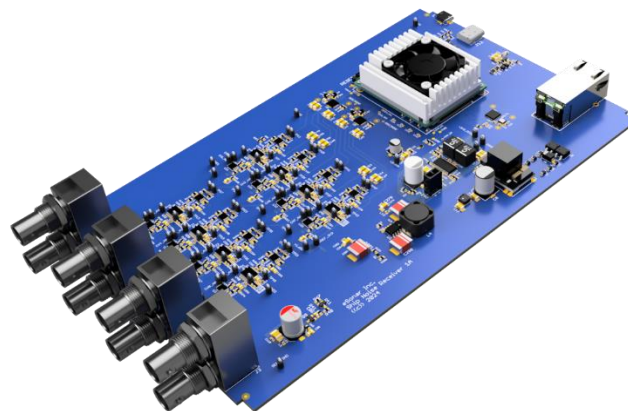
Figure 8-4 Printed circuit board model showing the placement of key components and PCB outline to fit the selected enclosure
