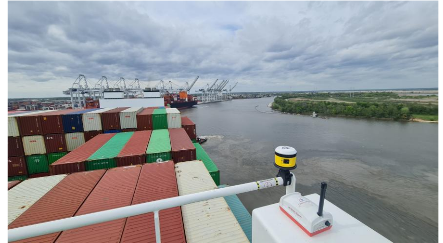
Measuring vessel motions near the berths
