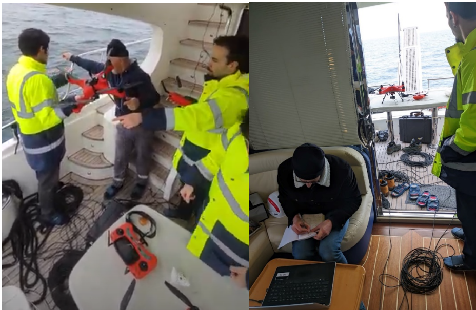
Figure 30: Deployment of both HyDrone and conventional array hydrophones from the support boat
