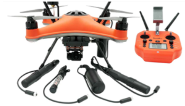
Figure 45: SD4 instruments for sampling and environmental monitoring
