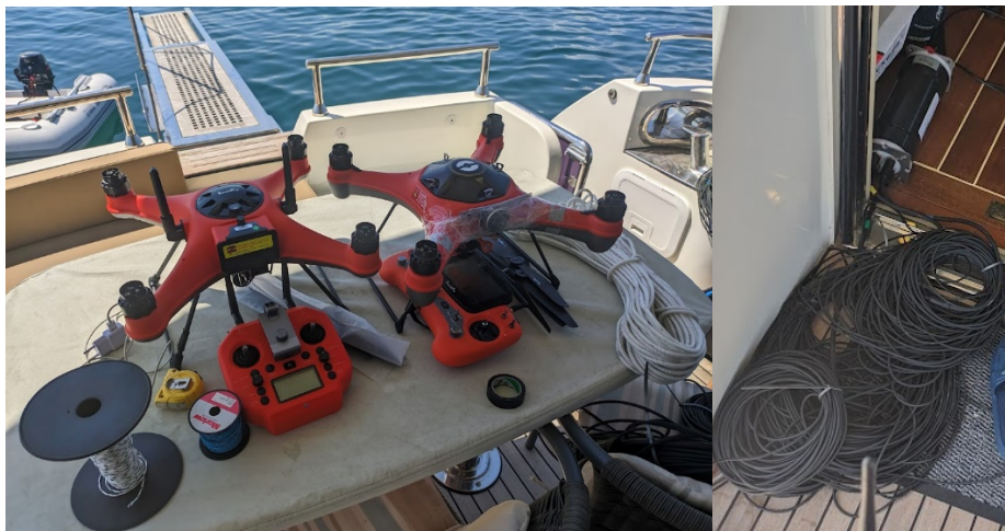
Figure 28: Deployment of both HyDrone and conventional array hydrophones from the support boat
