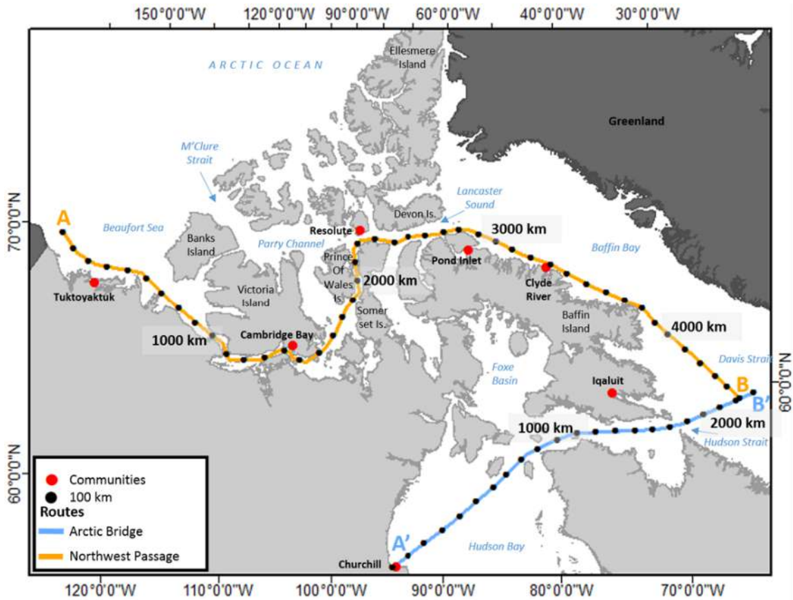
Map of the Northwest Passage primary shipping route (A to B) through the NORDREG zone, with 100 km markers, used to produce graphs of AIRSS values with distance.
